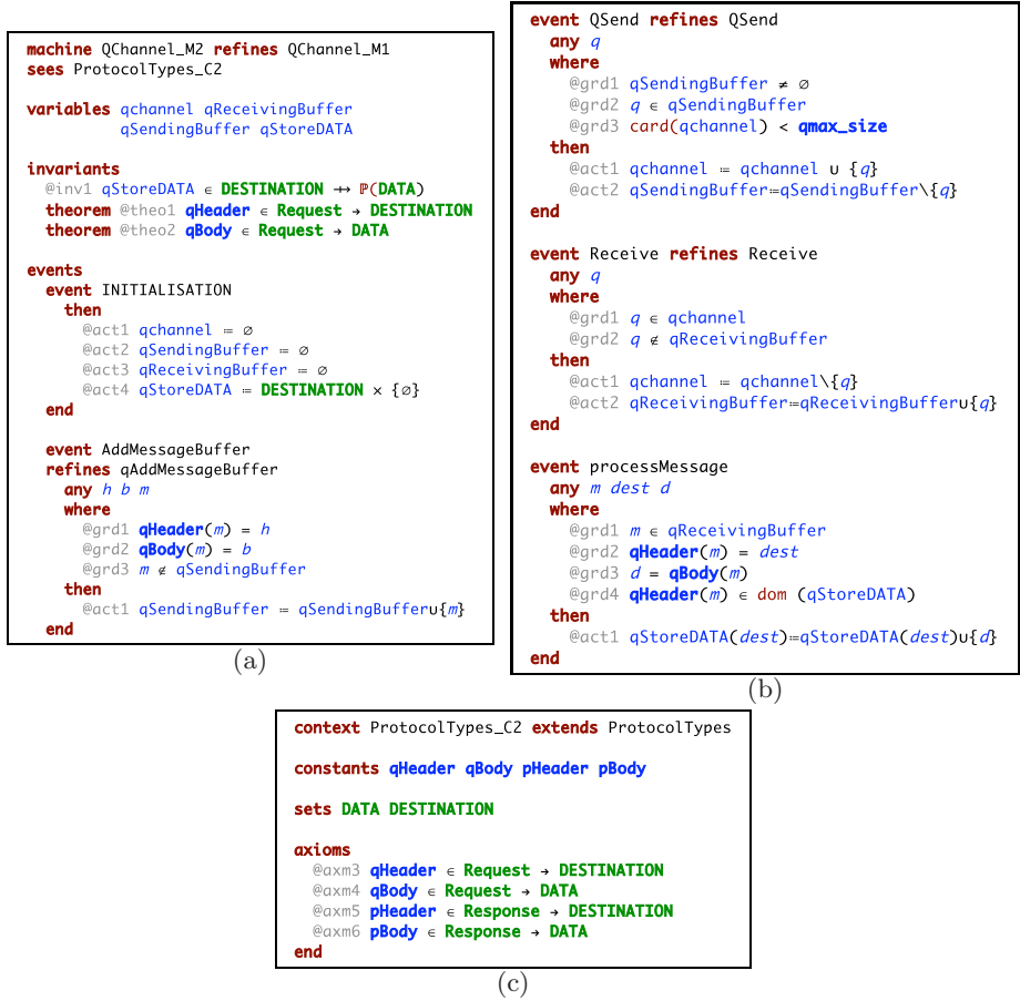
Fig. 16. Expanded version of instantiated machine QChannel_M2 and context ProtocolTypes_C2
