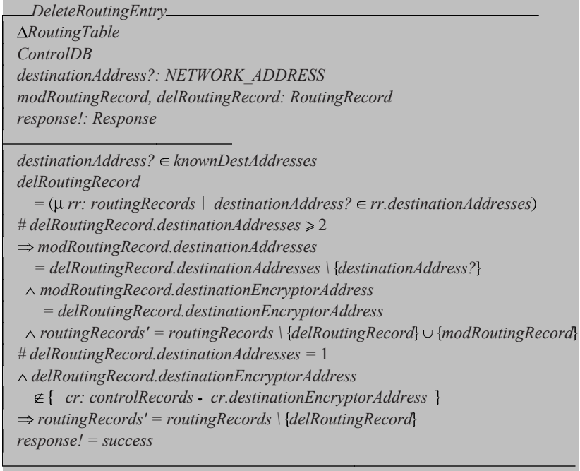
Fig. 12. Z Specification of DeleteRoutingEntry
